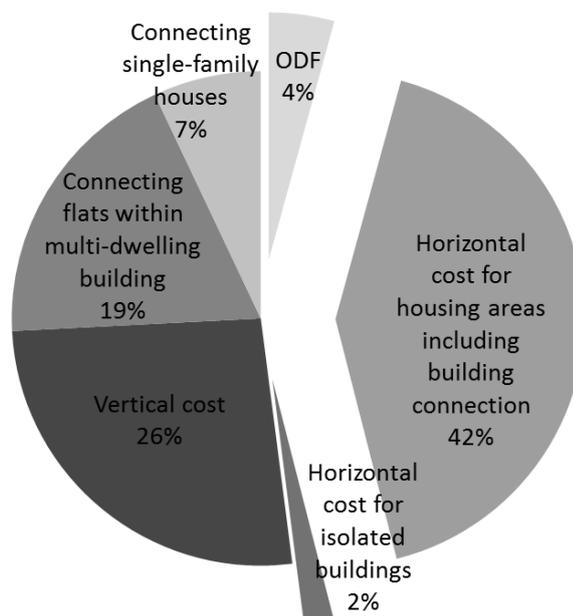
There is a factor that partially compensates for the cost increase following the duplication. It is the technological factor: PON technology is less expensive than the point-to-point one. Horizontal cost (study, supply and laying) excluding connecting buildings is higher by 20% in point-to-point.
