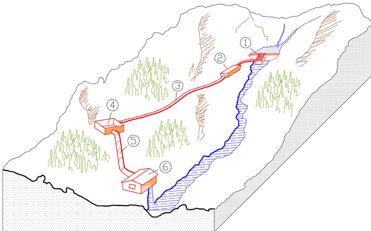
Figure 2: Main component of a high-head MHP plant<sup>15</sup>
