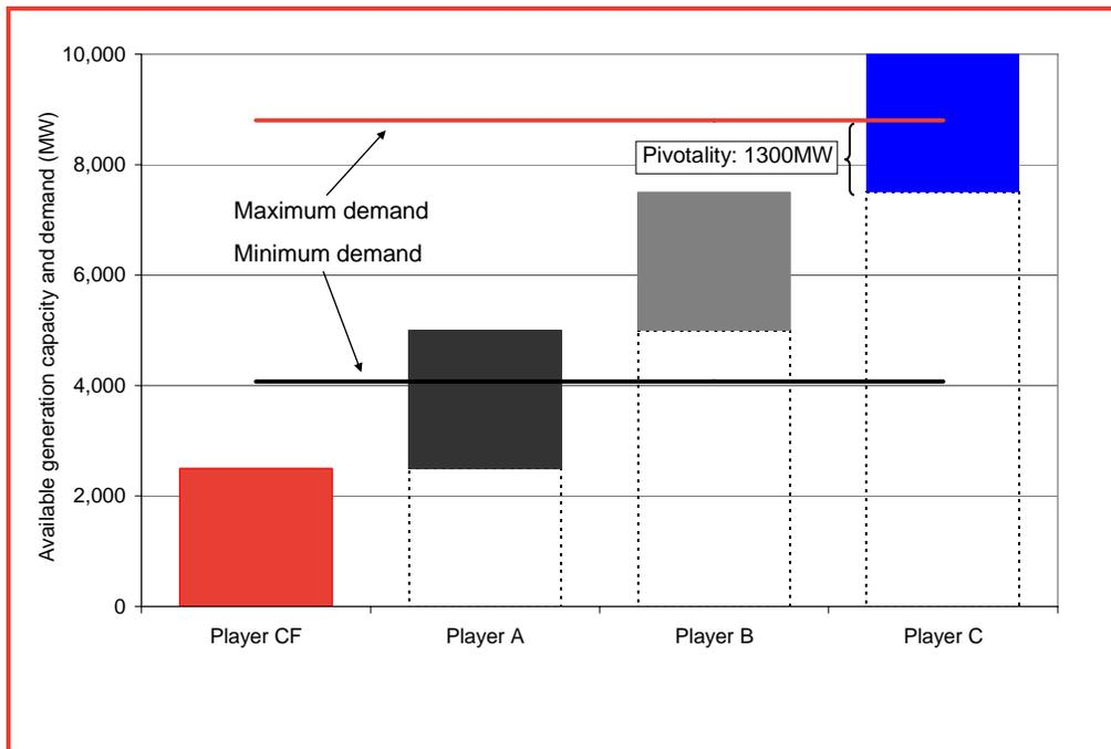
Figure 6: HHI capacity vs pivotal analysis (i) – low demand and small fringe.
