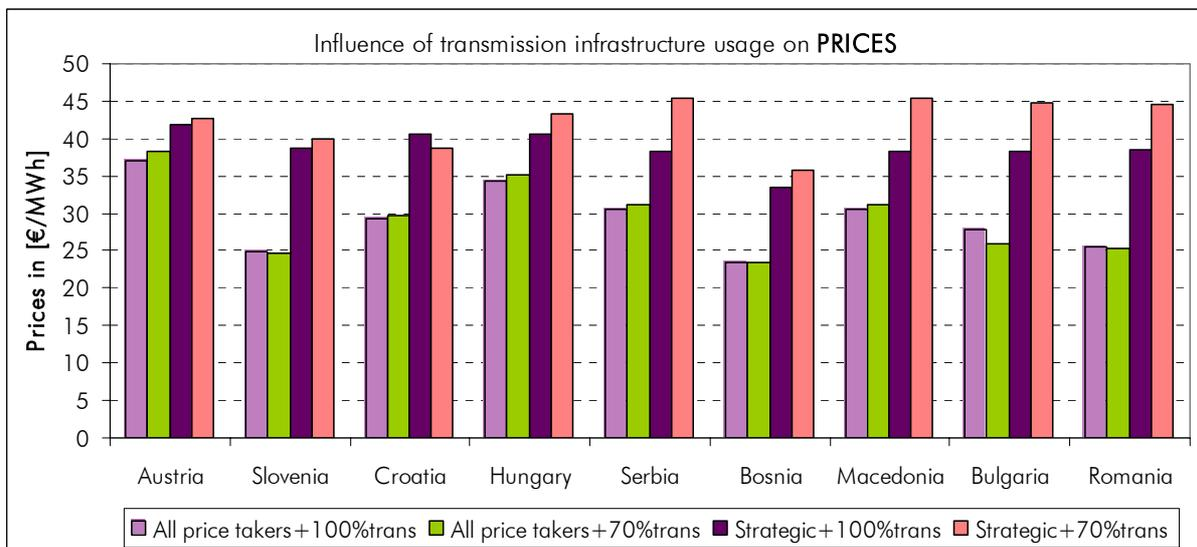
**Fig. 7. Influence of transmission infrastructure usage on prices (in €/MWh)**
