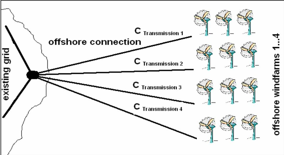
Fig. 1a. Separate offshore grid connection of each wind farm
