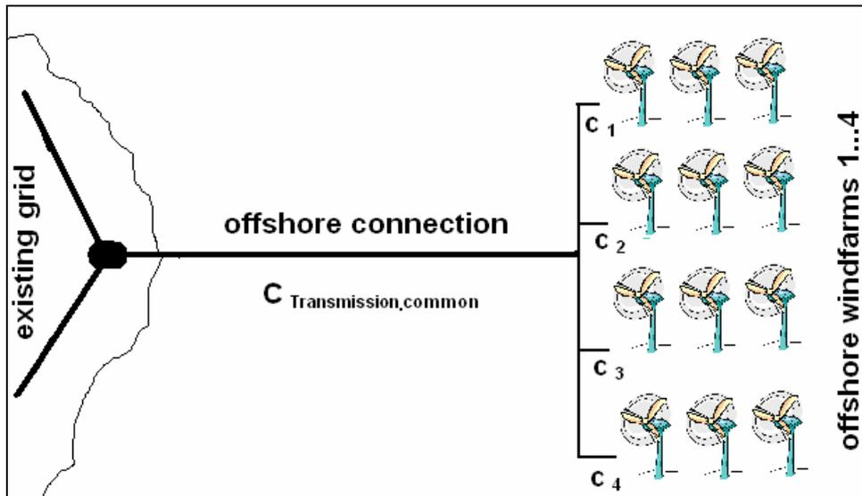
Fig. 1b. Common offshore grid connection of several wind farms
