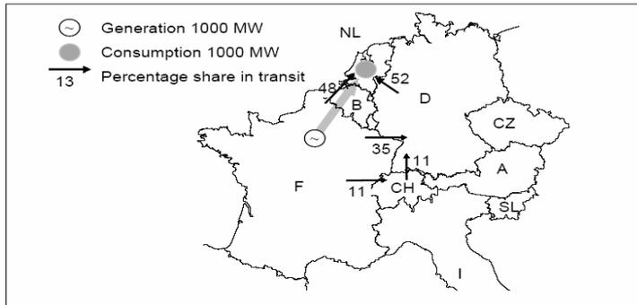
Figure 2: Power flow France Netherlands transaction (Haubrich, Fritz, Study on cross border electricity transmission tariffs, Aachen 1999, p. 13)
