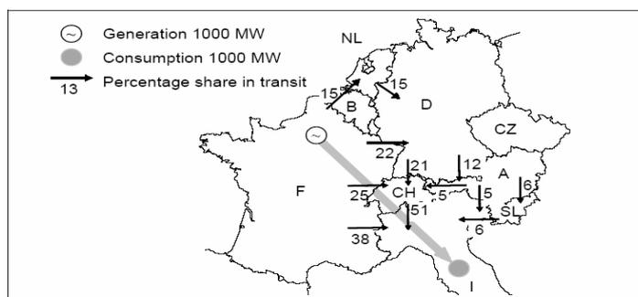
Figure 1: Power flow France-Italy transaction (Haubrich, Fritz, Study on cross border electricity transmission tariffs, Aachen 1999, p. 13)
