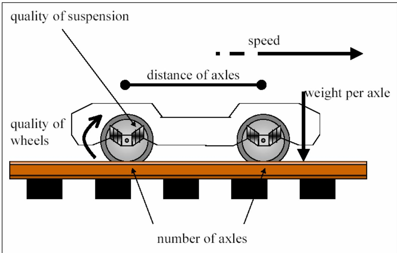
Fig. 1: Wear of rail caused by trains.
