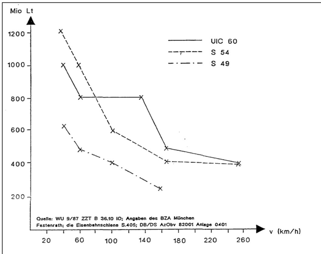
Fig. 2: Decreasing capability (in Tonnes) of rail in dependency to speed (Schroeder-Baumgart, 1993, p. 18)
